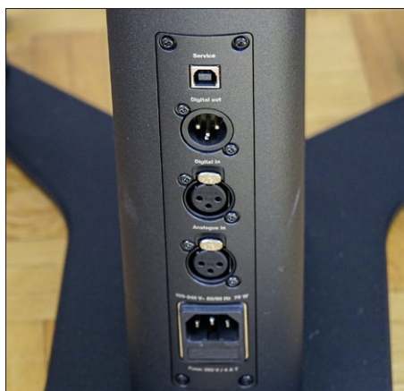
The connection panel offers analog as well as digital three-pin XLR connectors.
