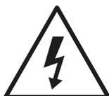
The lightning flash with an arrowhead symbol within an equilateral triangle, is intended to alert the user to the presence of uninsulated “dangerous voltage” within the product’s enclosure that may be of sufficient magnitude to constitute a risk of electric shock to persons.
