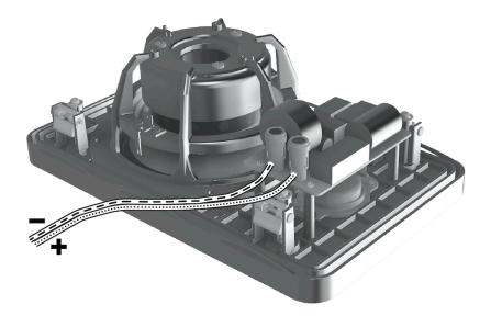
With the Speaker Unit connected to the speaker cable it can be inserted into the Installation Frame. Turn the locking tabs on the front surface of the Speaker Unit fully clockwise (aligned with the lock icons) and insert it in the Installation Frame. Push gently around each locking tab until a click is heard. The Speaker Unit will then be secured in the frame.
